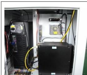
Inside of fiber laser marking machine
